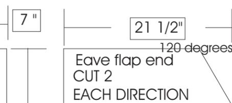
NOTE: The dimensions in the red boxes are higher than necessary, to allow for the entire top line to be cut after the end panel is assembled, cutting the excess off, thereby straightening the top line and cutting the height of the end panel to size. The final cut height of each end panel should be 36 inches at the low end (corner seam) and 72 inches at the high end (center seam). Note that this is the center seam, not the edge of the added door flap.
